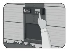
**2.9.** Press to test the door opening and closing.
