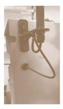
When using the external antenna outside the box, there is the same connection procedure and the same grommet for entering in the box.
